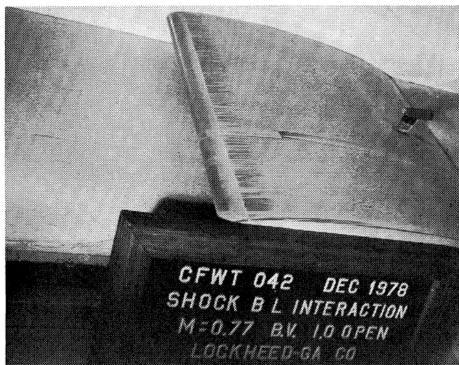
Fig. 10 Oil flow visualization at M = 0.78 , R_{N_c} = 11 \times 10^6 .
